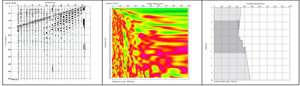
MASW Results from Line 3, Profile 18, Shot 5. From left to right images show the seismic shot record, the dispersion curve and the shear wave velocity - versus depth model.
