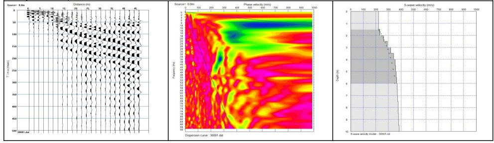
MASW Results from Line 5, Profile 24, Shot 6. From left to right images show the seismic shot record, the dispersion curve and the shear wave velocity - versus depth model.
