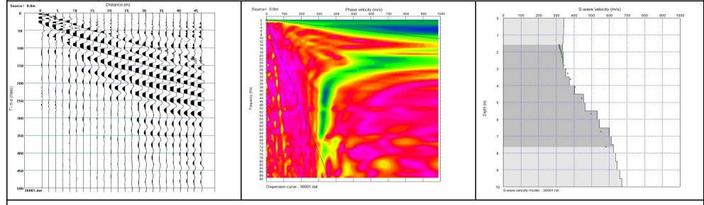
MASW Results from Line 2, Profile 9, Shot 5. From left to right images show the seismic shot record, the dispersion curve and the shear wave velocity - versus depth model.
